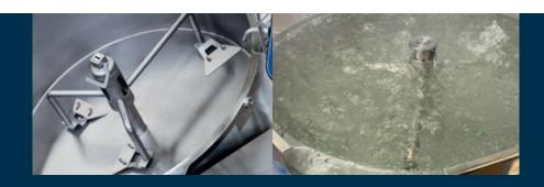
Direct heating while mixing allows rapid boiling of all liquids an Ali Group Company
