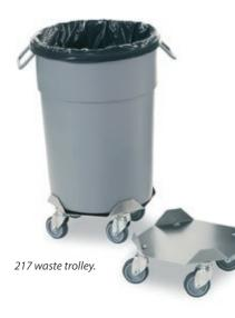
**Nordien-System waste trolley** in heavy duty design with rilsan coated handles. Convex bottom for easier emptying and cleaning. Diameter 385 mm and volume 45 litres. Separate stainless steel chassis is fitted with 75 mm ball bearing wheels, two with brakes.
